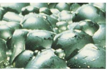
Molybdenite particles coat bubbles during flotation process
