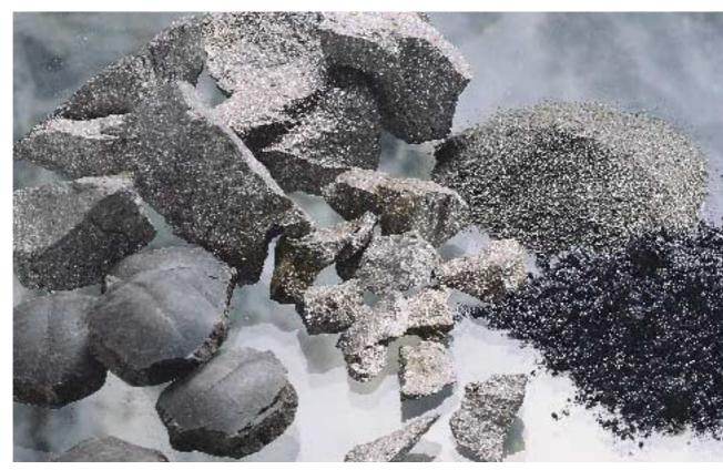
Samples of technical oxide and ferromolybdenum
