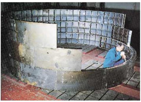
London Tube tunnel linings use highly alloyed super duplex stainless steel
