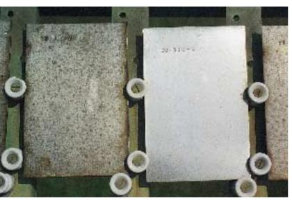
Types 304 (0% Mo) and 316 (2-3% Mo) test panels after 56 years marine exposure
