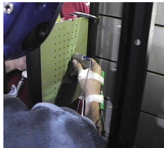
Figure 2. Accelerometer attached to the bucking bar during the experimental task.
